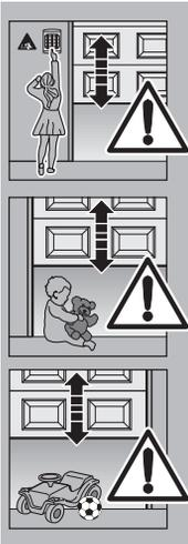
Permanently installed controls (such as push-buttons, switches etc.) have to be installed within sight of the door but well away from any moving parts at a height of at least 1.5 m. It is vital that they are installed out of the reach of children!
